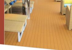
Syntheteak and Decoro are durable, decorative systems designed specifically for outdoor applications. Both are nominal 3/16 in. /5 mm resilient, aliphatic polyurethane flooring systems, designed for outdoor solutions for the hospitality industry pool decks, bars, patios and reception areas.
